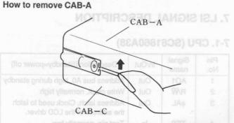
As shown in the figure above, insert your nail in the clearance between CAB-A and CAB-C near the hinge and push it down in the arrow direction to disengage the latch C at two locations (Fig.2).
