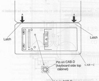
Hole in CAB-C (keyboard side bottom cabinet)
