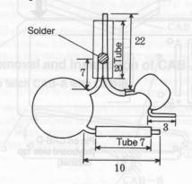
Provide the following 100Ω resistor.
